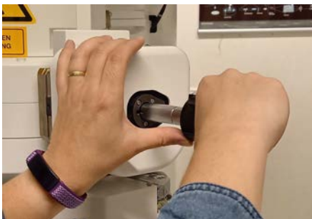
Figure 12: How to support the holder while inserting it into the TEM. One-handed: with the index finger. Two-handed: with the thumb of the left hand.
